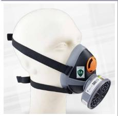
**Description:** Half mask in PP and TPE equipped with an adjustable elastic head harness in Dacron and Lactoprene and an exhalation valve in silicone. The half mask is equipped with one special bayonet connector including an inhalation valve in silicone (detailed description in EC type examination report 15.7.031.001) Materials: Half-mask: silicone Elasticated straps
